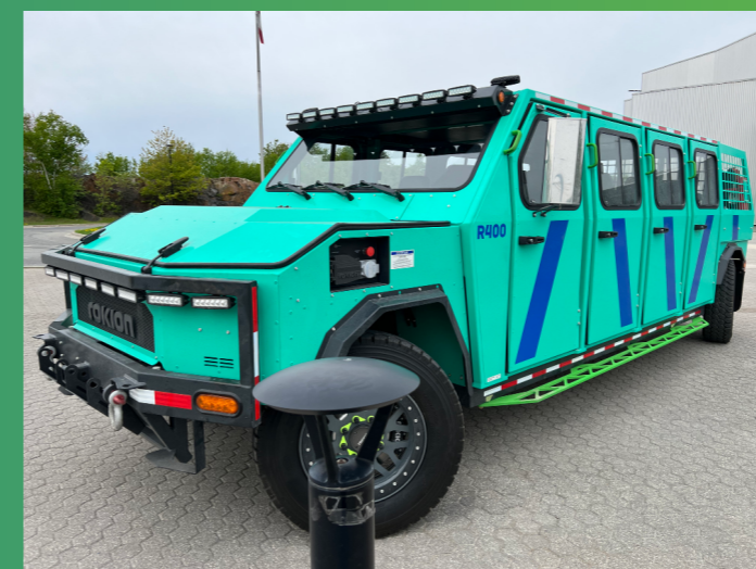
A Rokion underground battery electric personnel carrier on display at Science North in Sudbury, ON
